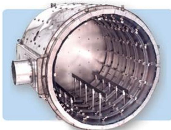
Shield packs are typically constructed from 3-5 layers of thin sheet (typically 0.03 to 0.06" thick). Both rectangular and cylindrical systems are used, in both horizontal and vertical configurations. These sheets are cut, punched and assembled using traditional sheet metal techniques. The sheets are
