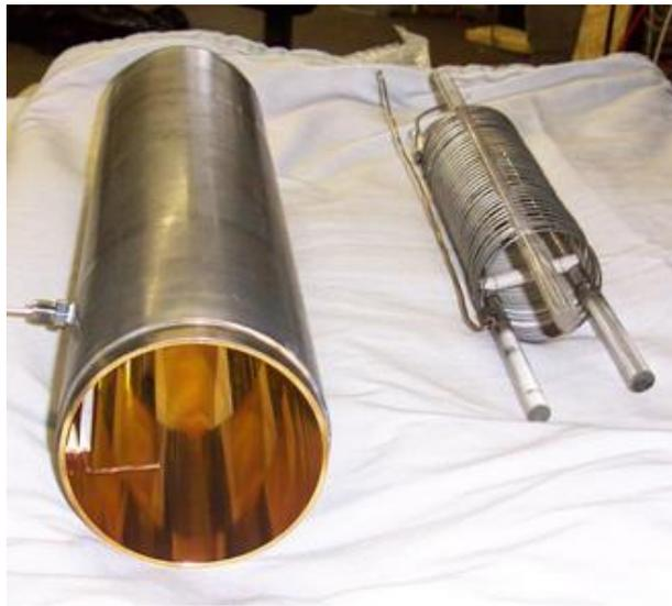
Figure 6. Photograph of gold plated low emissivity outer shell and coil assembly used in testing.
